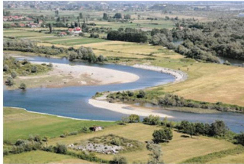
1.35 Meanders in the Kir River near Shkodër, Albania, show the classic pattern of point bars deposited on the insides of meanders, and erosion on the outsides of each meander. The meander in the centre of this photo has been reinforced by a stone wall to prevent further outward migration of the meander.
