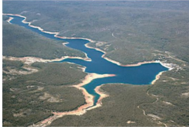
4.16 The reservoir behind Canning Dam near Perth, Western Australia, has a surface area of just five square kilometres, but this leads to an increase of evaporation in the warm, dry climate. exposed to the wind and sun lose more water than bare ground surfaces.
